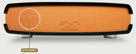
Turn on the amplifier from the rear panel IEC mains switch, then touch the front panel standby disk to enable the GaNFET amplifier modules (the light ring around the disk will illuminate). Touch again to put the amplifier into standby mode (the light ring around the disk will turn off). This disables power to the GaNFET amplifier modules.
